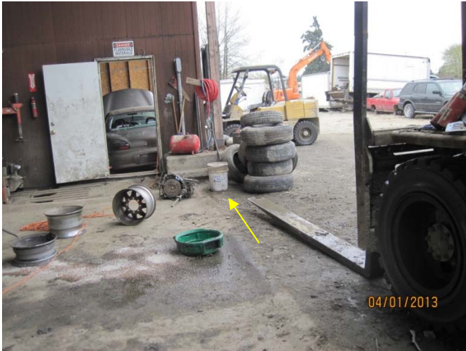
#7 DESCRIPTION: SPILLS ARE OUTSIDE THE SECONDARY CONTAINMENT AREA. ALSO, 5-GALLON CONTAINER PLACED OUTSIDE CONTAINMENT AREA.
